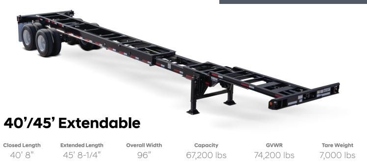
Durable and versatile, the 40'/45' Extendable features reinforcement bracing near the landing gear to redistribute the load evenly across the main beam. A locking pin release mechanism fully contained within the main beam protects against shearing. This model can carry a 40' or 45' container.
