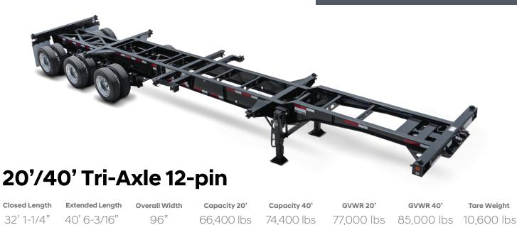
The 20'/40' Tri-Axle Combo Slider can handle a variety of configurations. A 12-pin design allows this model to carry one 20' container, one 40' container, or two empty 20' containers. The tri-axle configuration is built for heavy duty hauls and offers increased capacity compared to standard models.
